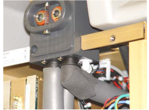
Inlet / Outlet Manifold
