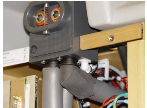
Inlet / Outlet Manifold
