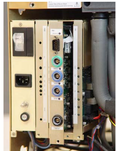
Isolation Circuit Card Figure 7.15
