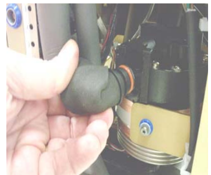
Removing Pump Port
