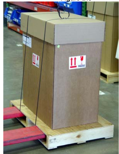
Packaged and Banded to Pallet Figure B.4
