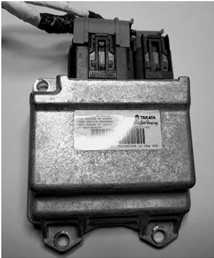
Figure 4-1: A typical event data recorder
